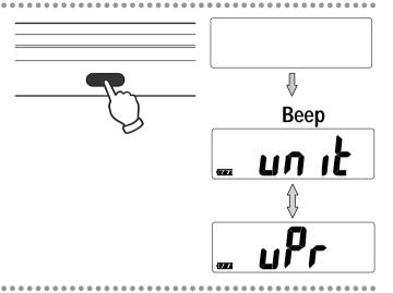
2. Release the setting switch when "uPr" is displayed.
