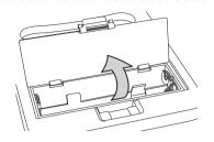
Install four new AA size alkaline batteries with the positive (+) and negative (-) terminals properly aligned with the corresponding symbols in the battery compartment.
