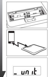
Install the batteries (P.5)
